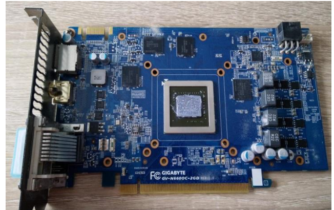
Graphic Card(VGA) – Heat Sinking Plane removed
