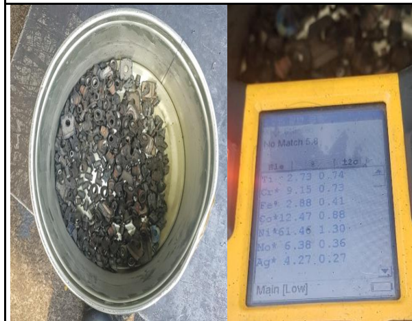
Disassemble Nut (Co, Ag, Mo Coating)
